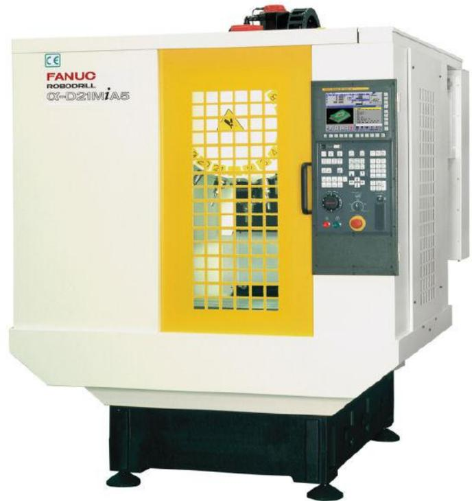
The new machine boasts an impressive 24,000 rpm High Speed Spindle, and 21 tool storage carousel, ideally suited for the variety of parts machined for the Medical Industry and for the civil and military Aerospace sectors.
